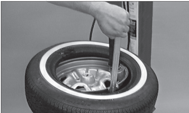
Figure 15 - Demounting Lower Bead
