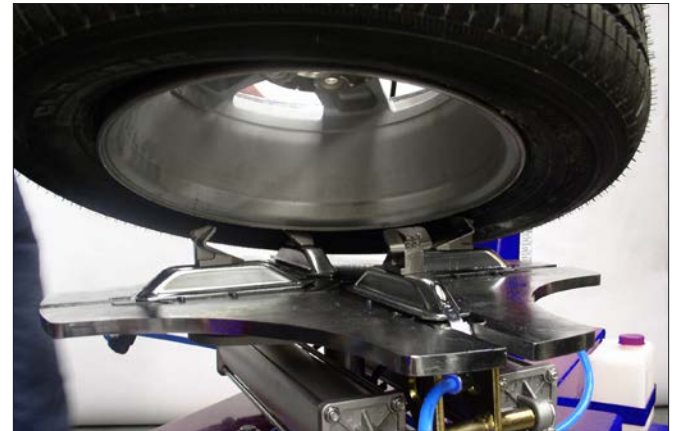
Figure 9 - Place Tire/Wheel Assembly on Table top
