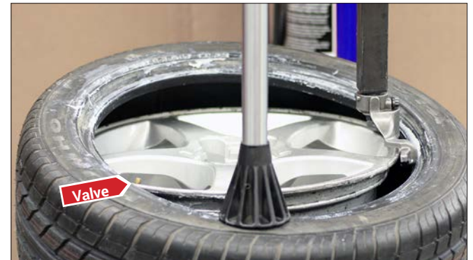
Figure 32 - Mount Upper Tire Bead, Use Helper Arm
