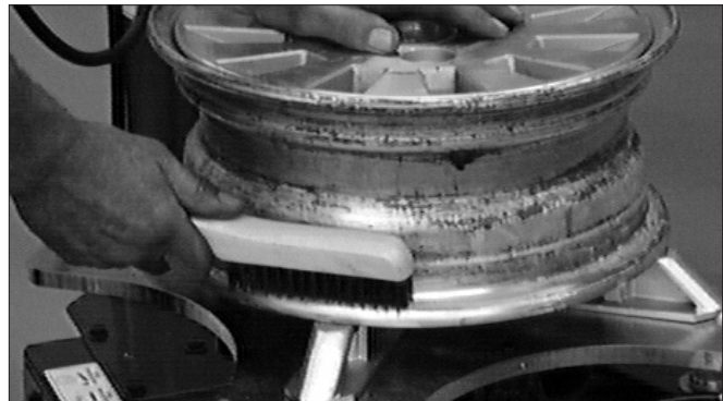
Figure 18 - Inspect and Clean the Wheel
