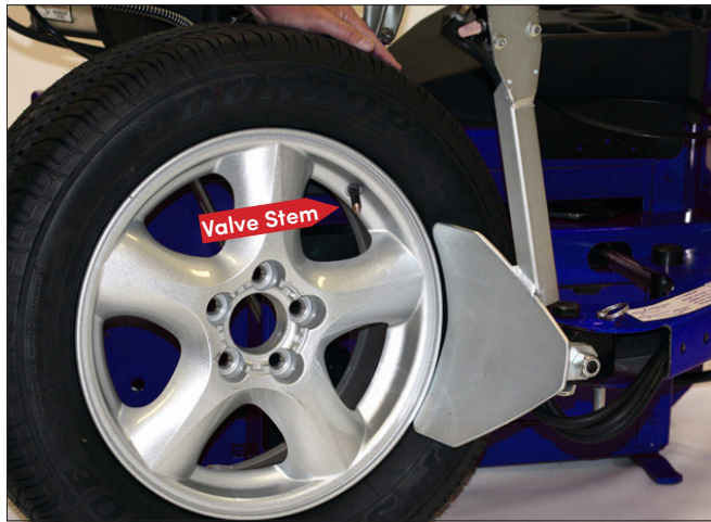
Figure 6 - Position Tire and Bead Loosener Shoe
