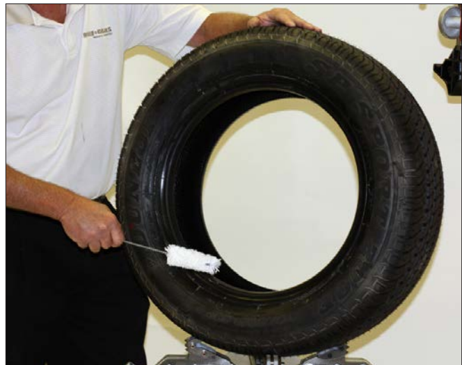
Figure 19 - Lubricate Tire Beads Liberally
