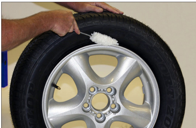
Figure 8 - Apply Rubber Lubricant to Tire Beads
