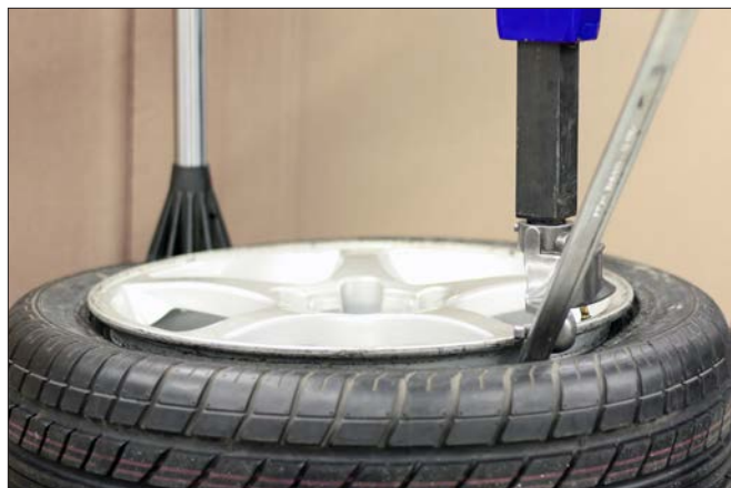
Figure 28 - Insert Bead Lifting Tool
