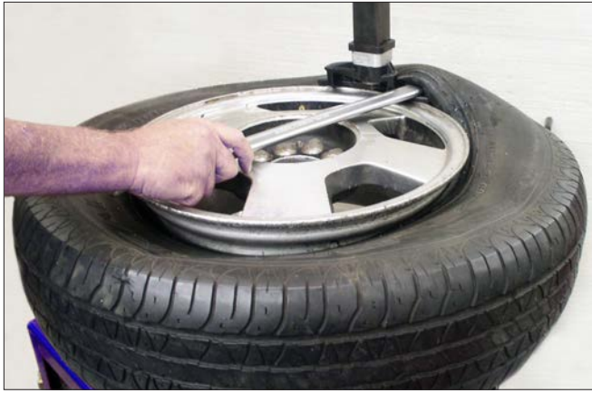
Figure 29 - Holding Lifting Tool in Place and Rotate Wheel
