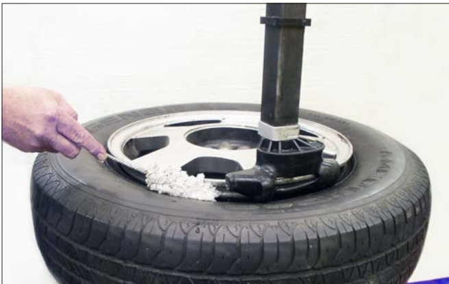
Figure 26 - Lubricate Upper Bead
