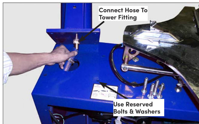
Figure 2 - Assemble tower onto chassis.
