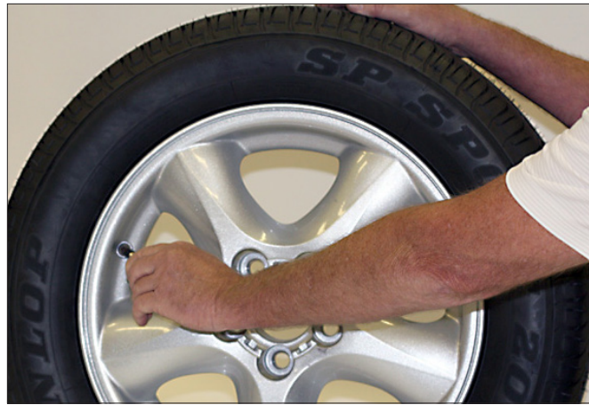
Figure 4 - Remove Valve Core to Deflate Tire
