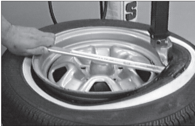
Figure 14 - Lift Tire Bead Over Duckhead® Mount/Demount Tool Knob
