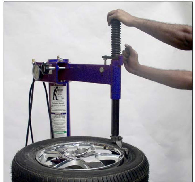
Figure 10 - Position Mount/Demount Tool.
