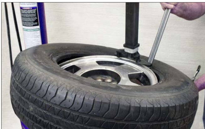
Figure 31 - Lower Tire Bead in Drop Center
