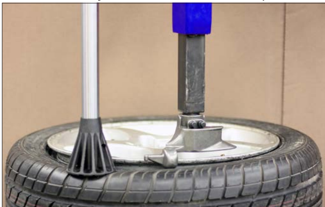
Figure 25 - Helper Arm Foot Depressing Sidewall of Tire
