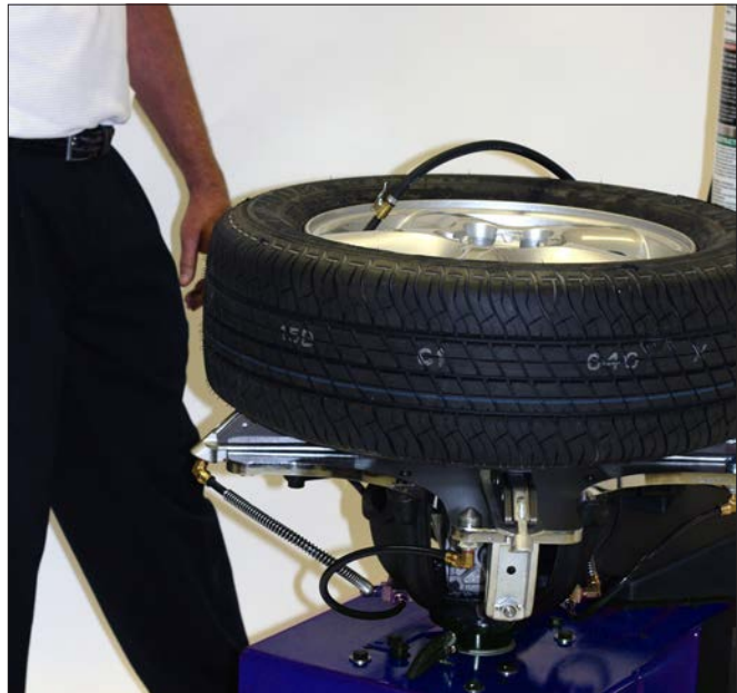
Figure 23 - Stand Back during Bead Seat
