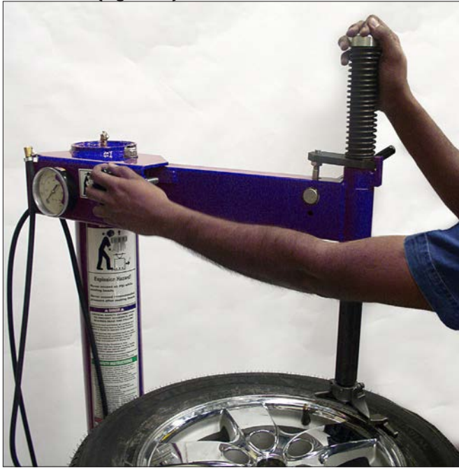
Figure 11 - Adjust Swing Arm to Position Tool Roller
