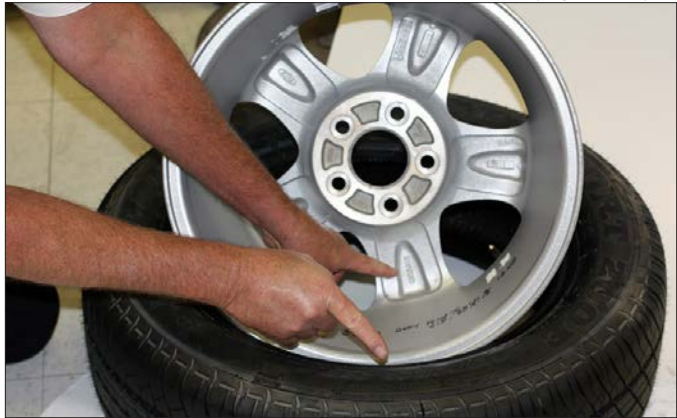
Figure 17 - Verify Size Match Between Tire and Wheel
