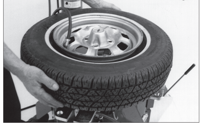
Figure 22 - Lift Tire Upwards for Bead Sealing
