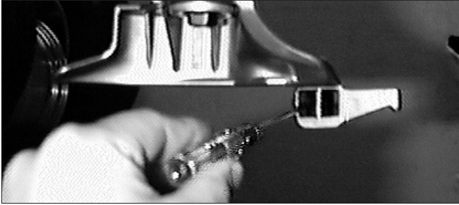
Figure 34 – Clean Duckhead® Mount/demount Tool Using Small Screwdriver
