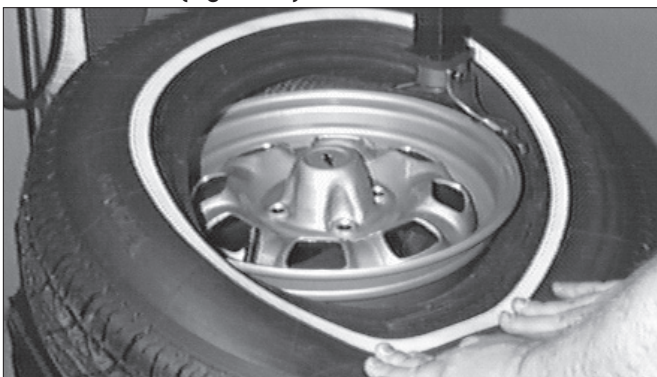
Figure 21 - Mounting Top Bead
