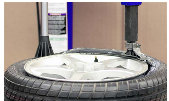
Figure 33 - Helper Arm Foot to Flip Bead Over Rim Flange
