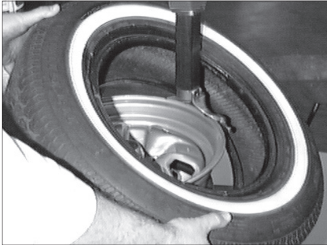
Figure 20 - Position Tire Against Mount/Demount Tool
